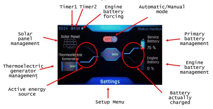
This menu shows the status of the system in terms of energy management. It clearly indicates which energy source is charging which type of battery. It shows the actual mode of operation (manual or automatic), the charge level of the batteries, the status of the timers and the possible forced recharging for the engine battery.
