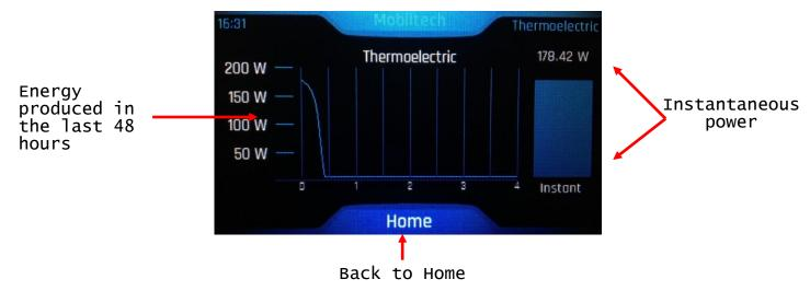
The graph shows the trend of the energy delivered by the thermoelectric generator over the last 48 hours. Touching the graph area, a zoom is performed in order to view the progress of the energy generation more accurately. On the right side is shown the energy produced instantly, both graphically and numerically
