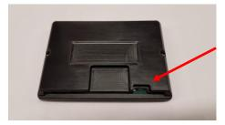
The update is performed by inserting a memory card with the new software package into the MicroSD slot.
