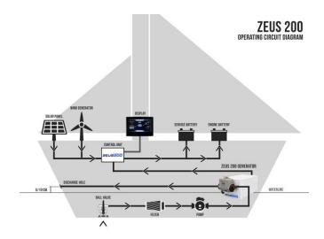
Zeus200 generator is able, using the boat fuel, to charge and maintain charged both the engine and service batteries. It is able to supply 200W of typical power; it's able to manage also an optional photovoltaic panel/eolic generator, preferring renewable sources when available.
