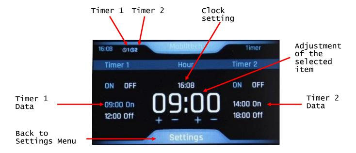
In this menu it is possible to activate, deactivate and adjust the on-off times of the two available Timers, as well as the internal clock. To set a timer, press the related time and make the desired adjustments in the central part of the screen. When the two timers are activated, the related icons on the main screen light up.
